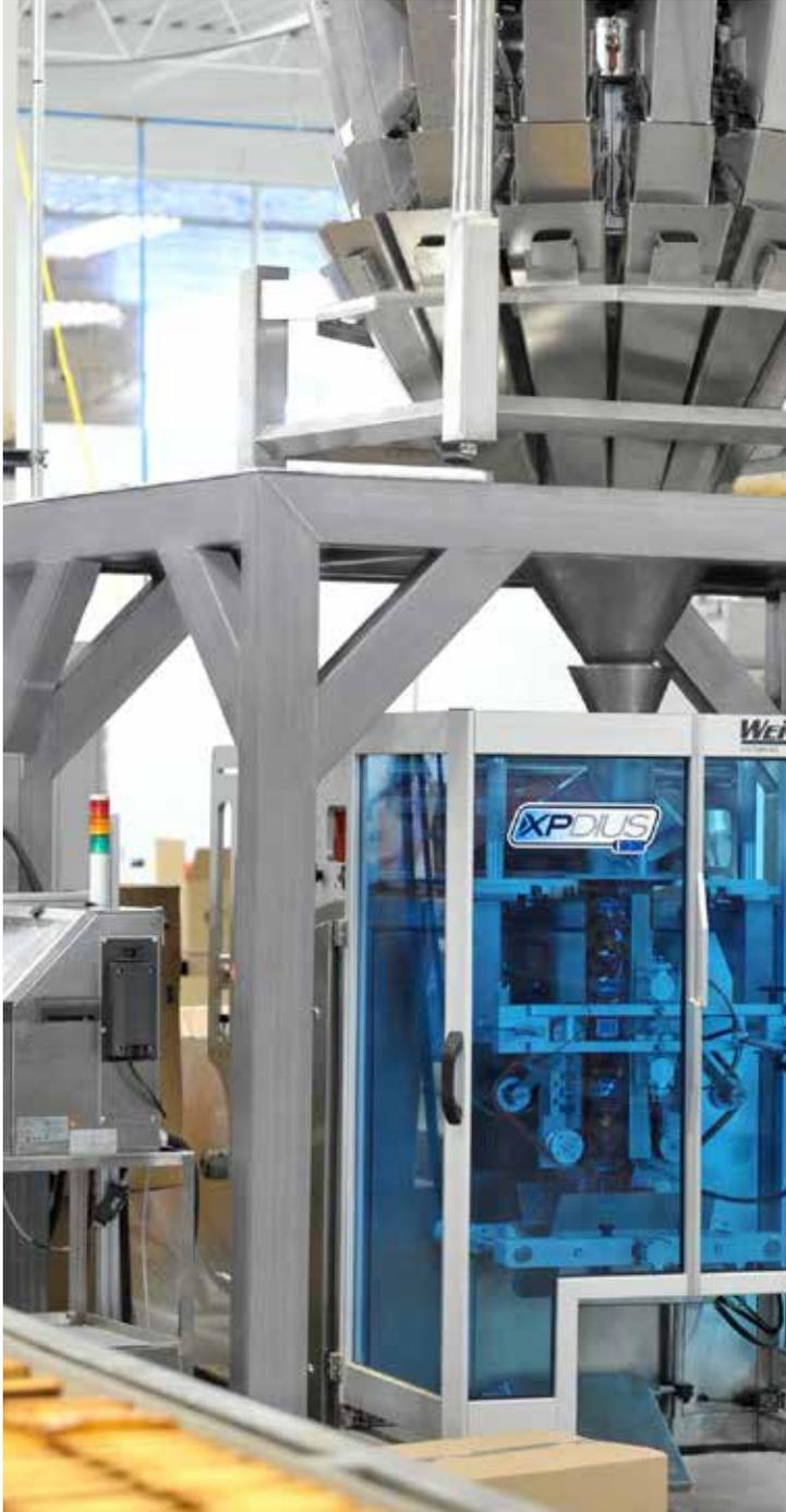
Our heavy duty floor stands are engineered to support a filling machine above a packaging machine. While they look simple, they are designed for optimal weight distribution, vibration control and include high quality welding and polishing.
